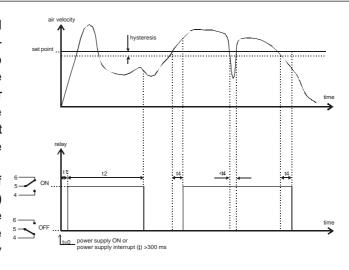
Only after that the air velocity switch reacts to the TRUE and RATED VALUE. The reaction time is limited by the response time ( $t_4$ ) of the sensor probe which is about 2 s. The described function is related to continuous operation, which is reached after a warm-up phase of approx. 3 min after applying the supply voltage.
